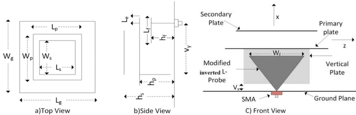
Figure-1. Geometry of proposed SSPA.
