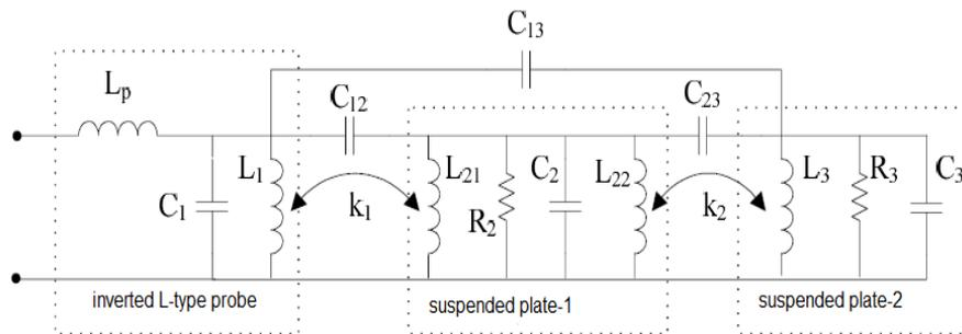
Figure-3. Equivalent Circuit of SSPA
